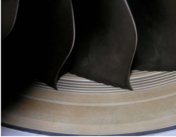
Figure 6.—Closeup of FML Installed OTR.
