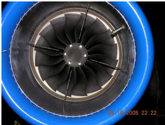
Figure 18.—Photo of Inlet Steady-State Pressure Instrumentation.
