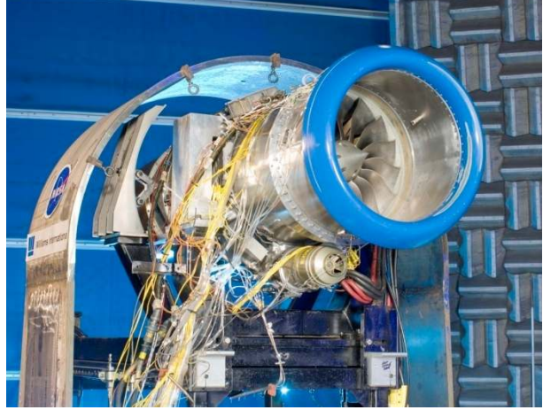
Figure 7.—FJ44 on Test Stand in AACL.
