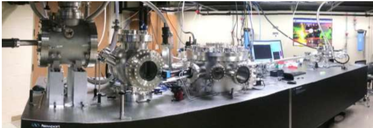
Figure 5.9. Attosecond-pump attosecond-probe endstation as installed at UCF.
