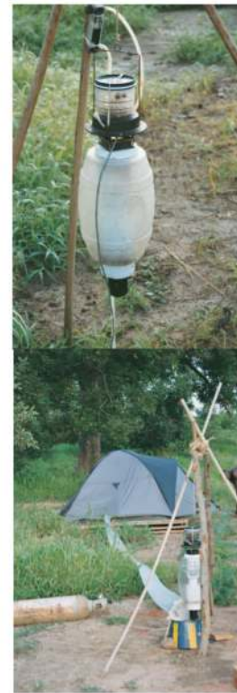
Fig. 1. Schematic drawing of the MM-X (alias Counterflow Geometry) trap (after Kline 1999) with an extra stimulus container. The top photograph shows the MM-X trap, and the bottom photo shows how odors from a human occupied tent were led to the MM-X trap via lay-flat tubing.
