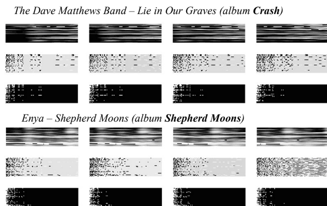
Figure 1. The representation for two songs – 4 consecutive spectrogram images shown for each, skipping 200 ms. For each song, top row: original spectrogram image, second row: wavelet magnitudes; third row: the top-200 wavelets. Note that the top wavelets have a distinctive pattern for each of the songs.
