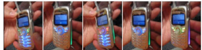
Figure 1. An example of moving information off the screen space. The e380 phone has tri-color sidebands and vibration to light up and shake depending on ringtone.
