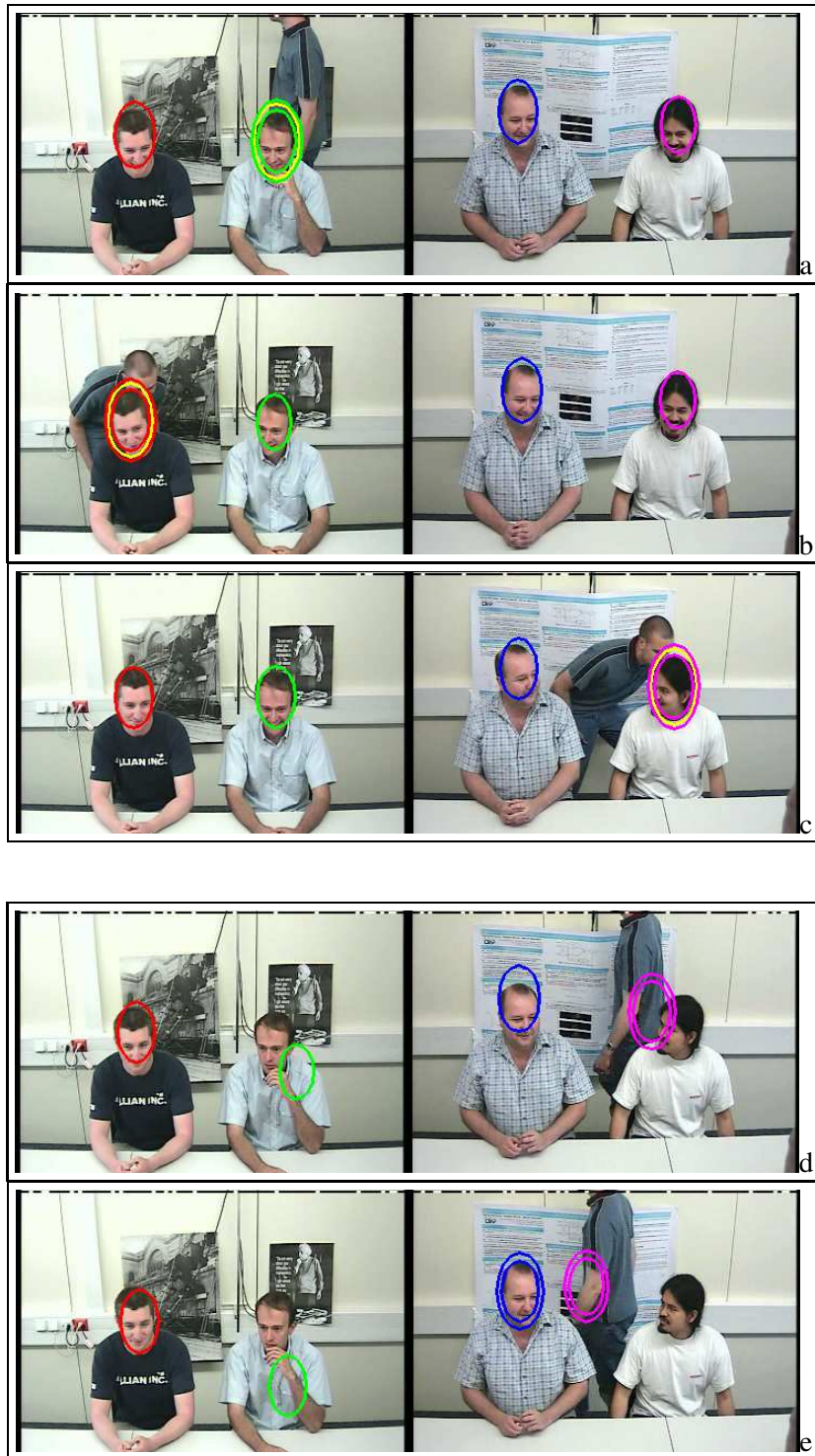
Fig. 5. Multispeaker tracking results, meeting2 . (a-c): MCMC-PF, images correspond to frames 360, 575, and 909, respectively. (d-e): Traditional PF: images correspond to frames 195 and 200, respectively. Tracking is lost for O2 and O4 for the rest of the sequence.
