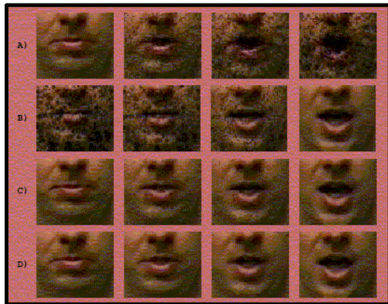
Figure 10: MikeTalk computes and blends two optical flows in order to symmetrically morph between two visemes
