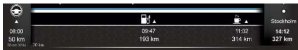
Figure 3. A design concept from the project MODAS [50]. A visual timeline (blue line) presented at the top of the windscreen indicates when a handover may be necessary.
