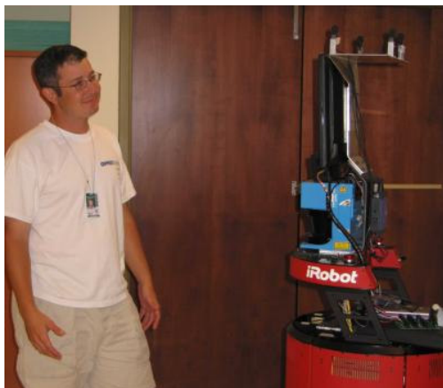
Figure 1. The robot is localizing a human speaker by their speech. The microphone array used in this task can be seen mounted at the highest point on the robot..
