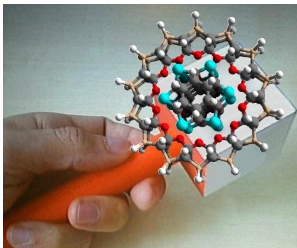
Figure 1. A hand held device is tracked by the Augmented Chemical Reactions application and visualizes a virtual molecule on top of it.
