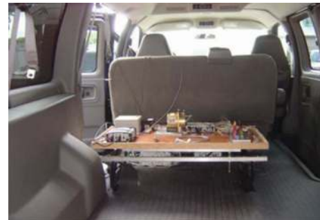
FIGURE 15: Data collection equipment mounted inside the road test vehicle.
