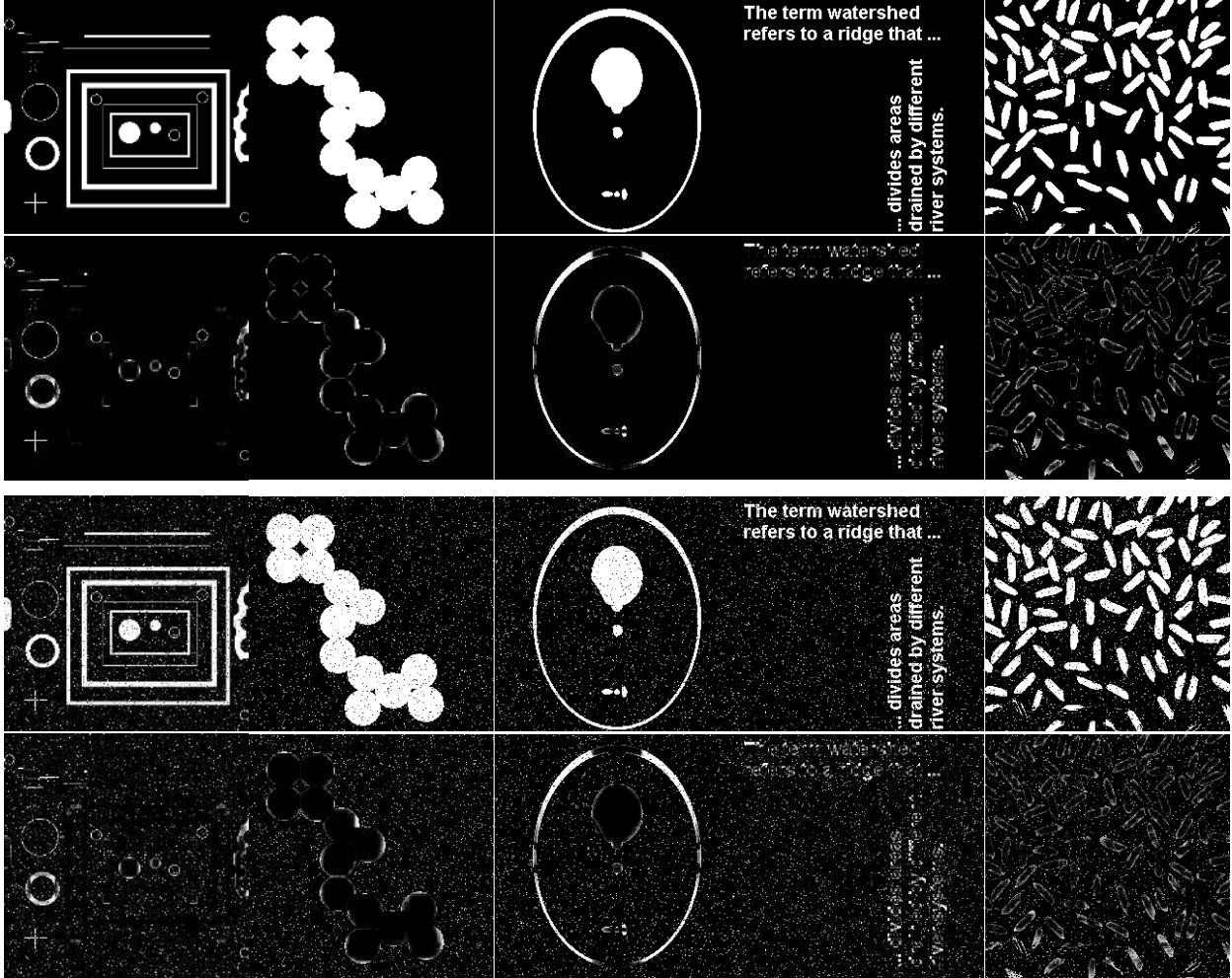
Figure 8: Recovered sparse images by LMaFit (the first and third rows) and IALM (the second and fourth rows). In the last two rows, impulsive noise is added to 10% pixels at random in each sparse image.
