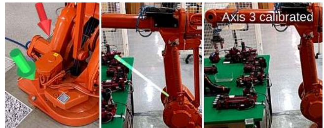
Fig. 5. Various types of specific point highlight visualization on the robot. In the left image the point is highlighted by 3D arrows. In the middle image the point is highlighted by leading line going from the left side of the screen to the down right point. In the right image the point is not directly highlighted but the state of the point is shown by text message.
