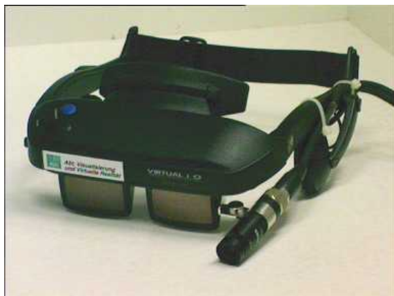
Figure 2: Head-mounted display with camera
