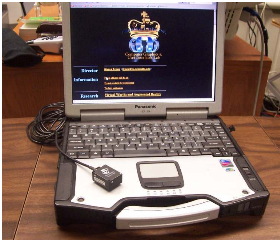
Figure 8. InterSense InertiaCube3 hybrid inertial-magnetic tracker
