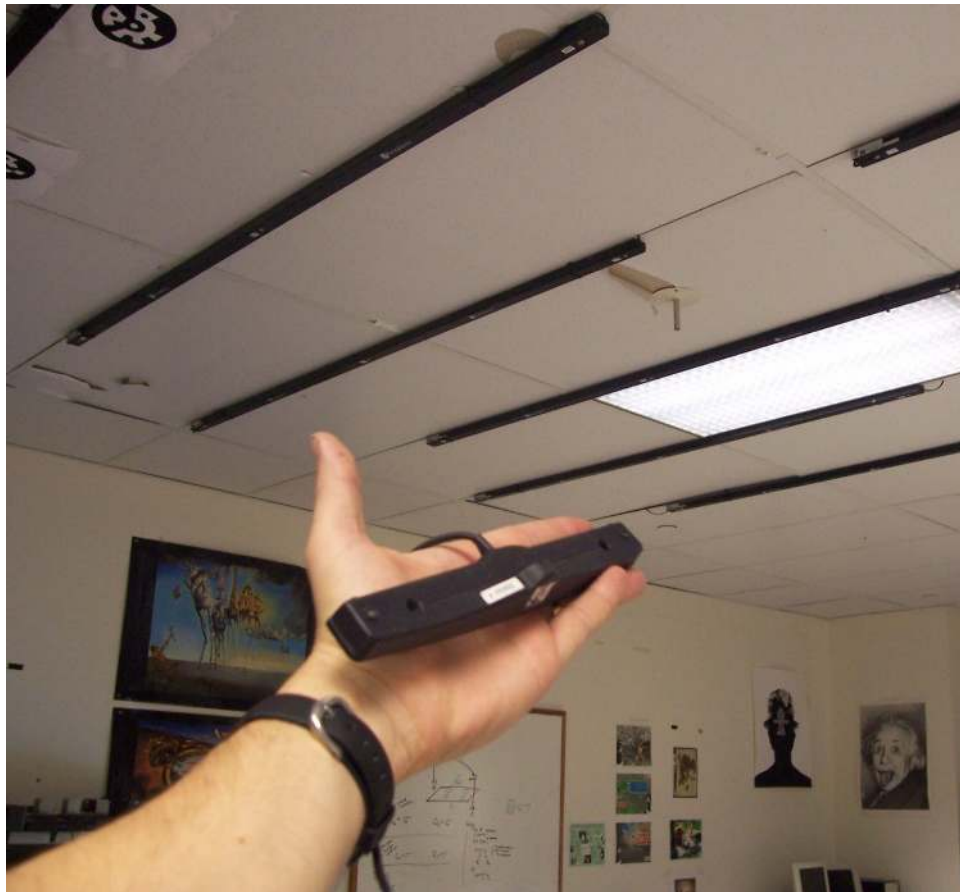
Figure 9. InterSense IS-900 hybrid inertial-acoustic tracker
