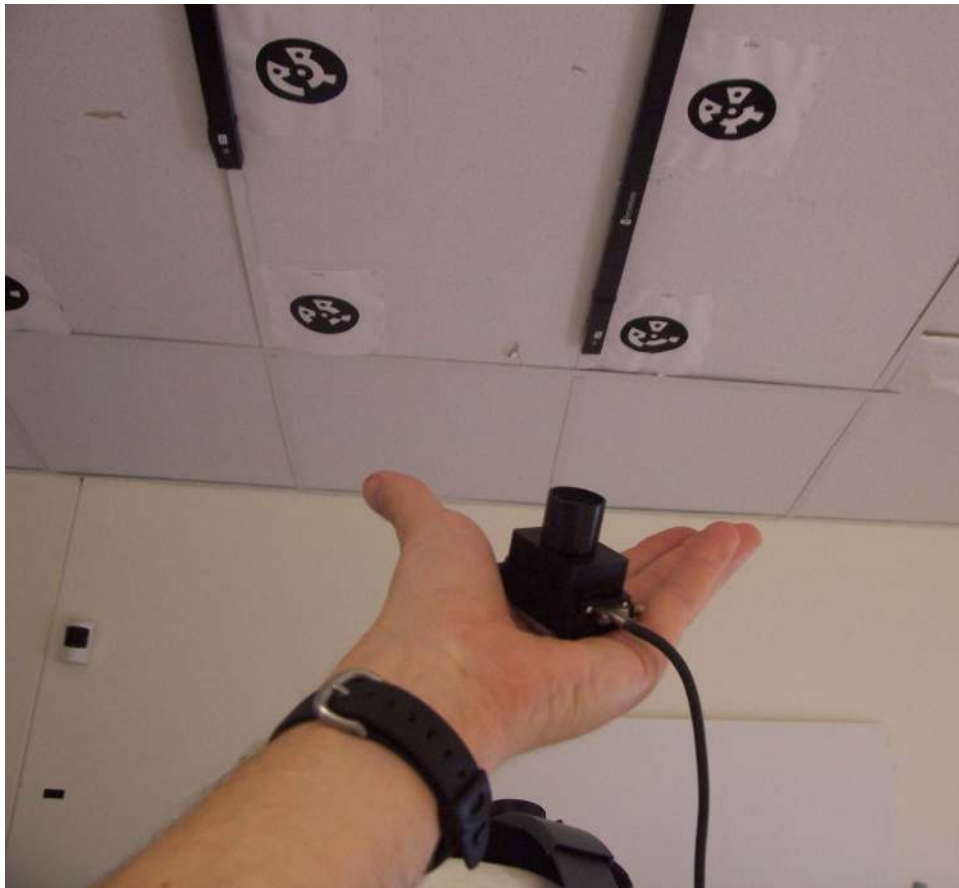
Figure 10. InterSense IS-1200 (beta) hybrid inertial-optical tracker
