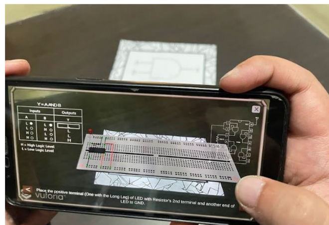
(f). LED is off when the user selects (LOW, LOW) as the input in AR application
