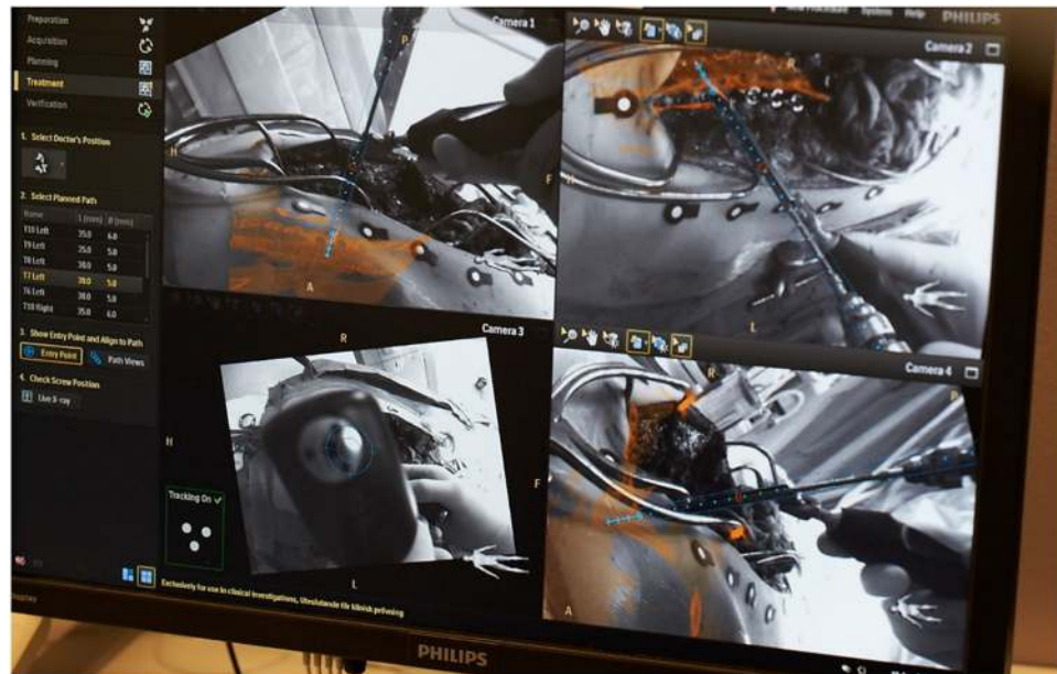
Figure 2. The surgical interface during navigated surgery is depicted. Each quadrant shows the surgical area at an angle, with the suggested instrument path in blue and underlying bone anatomy superimposed on the skin.
