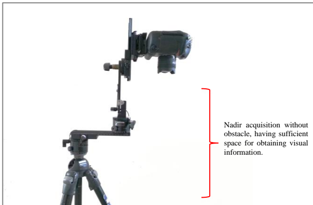
Figure 2: Camera mounting system that allows nadir acquisition.
