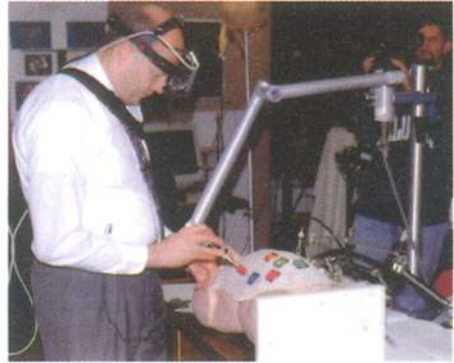
Fig. 2. The physician (Meyer) uses the system in the preliminary experiment (Dec 96). The mechanical arm he holds is unnecessary in the current implementation. The colored circular landmarks on the "body" surface assist the head tracking subsystem.
