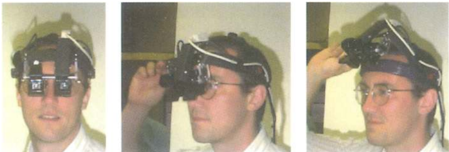
Fig. 3. (Above) Custom-designed video-see-through head-mounted display for augmented reality applications. The lightweight unit can be flipped up and down.
