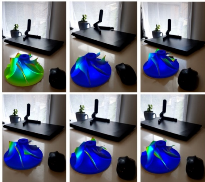
Figure 10. Modal analysis simulation results for modes 1 to 6 on the mobile AR visualization.
