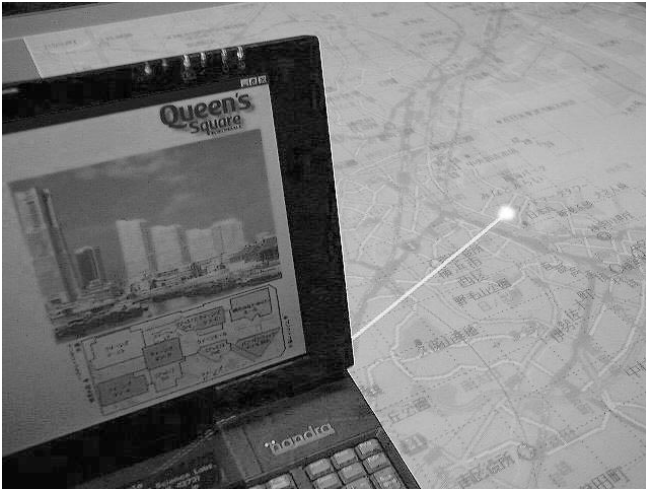
Figure 5: The anchored cursor shows the link between information on the table and the notebook computer
