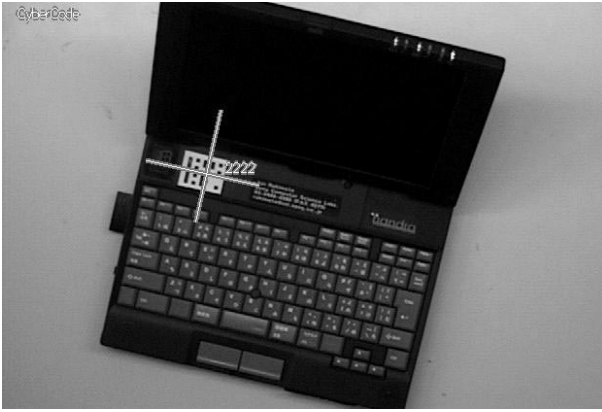
Figure 9: Visual marker recognition and obtained position and orientation.
