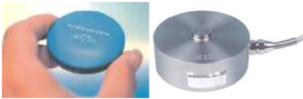
Fig. 4 The RF transmitter placed in a portable object like a key fob to detect presence ( left ) and the load sensor used under each leg of the bed to capture weight and sleep patterns ( right )
