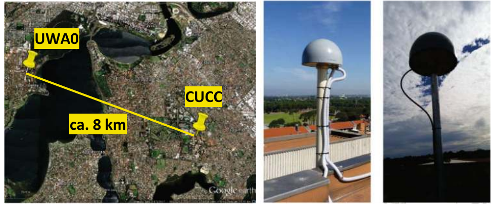
Fig. 3 Long baseline configuration. [Left] Baseline CUCC–UWA0 located in Perth, Australia. Map data @ 2018 Google (Google Earth 2018). [Middle] CUCC station. [Right] UWA0 station
