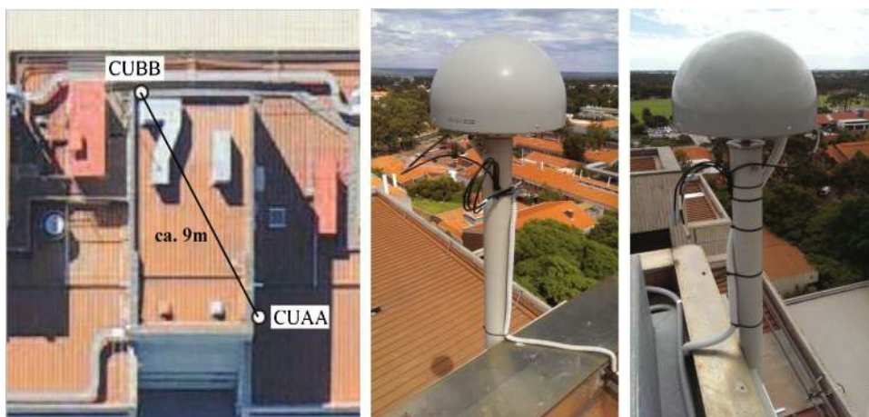
Fig. 2 Short baseline configuration. [Left] Baseline CUA A–CUBB located in Curtin University, Perth, Australia. [Middle] CUA A station. [Right] CUBB station
