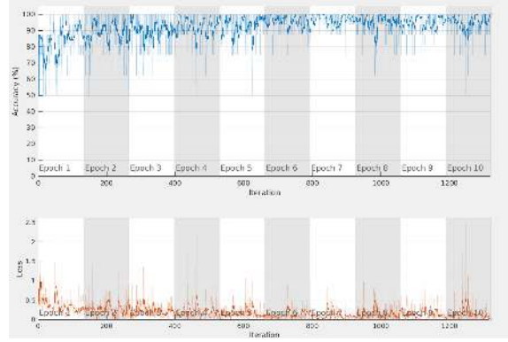
Figure 4: Convergence of the proposed semi-supervised shallow neural learning model allowing maximum 10 epochs during training with learning rate=0.001.
