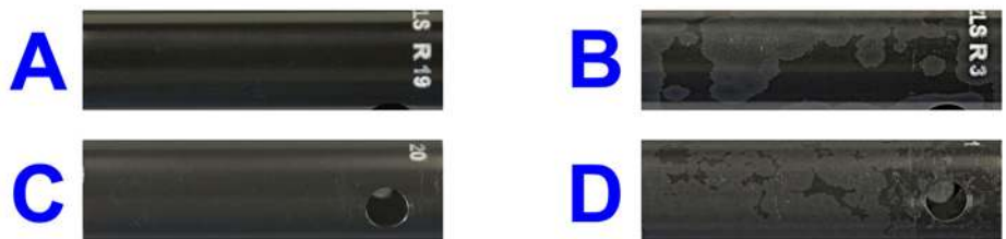
Figure 7: Autoclave corrosion weight gain profile of non-hydrated ZIRLO SR and RX materials. Photographs of actual corrosion specimens included: (A) non-hydrated ZIRLO – SR after 60 days of autoclave exposure, (B) non-hydrated ZIRLO – SR after 140 days, (C) non-hydrated ZIRLO – RX after 80 days and (D) non-hydrated ZIRLO – RX after 160 days.
