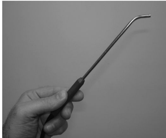
Fig. 2. Diagram and photograph of the clinical ball lens coupled fiber-optic probe.
