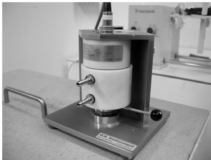
Figure 3.1 – Rotronic station for RH measurement
