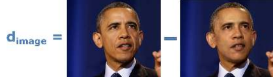
Figure 2: The image distance is computed by subtracting the input image with a modified version where the reconstructed face is rendered on top of the original face.
