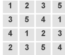
Fig. 4. A 5-pin layout for a 4 \times 4 array.
