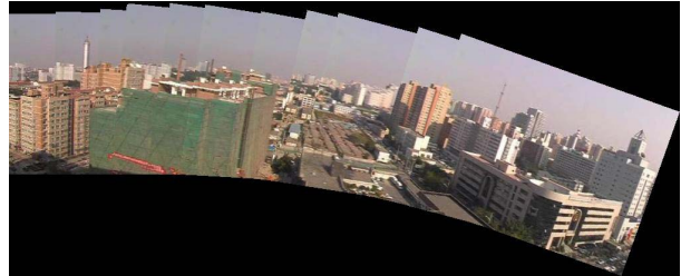
Figure 4. Mosaicing result from an input video sequence. 11 key frames are selected from 635 frames of the video sequence.
