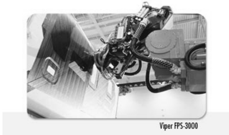
Figure 1: Photograph of Viper Tow Placement System (courtesy of Cincinnati Machine)
