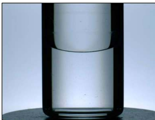
Figure 7. Image of an 8 mL vial showing the organic (top) and aqueous (bottom) phases.
