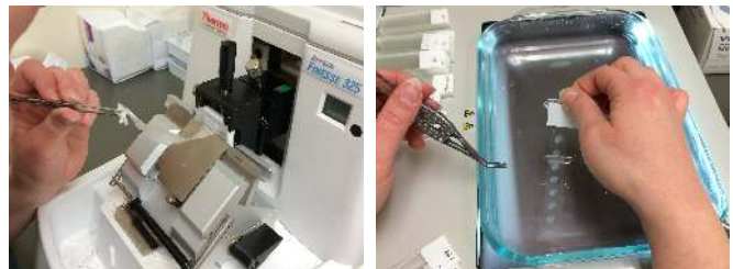
Fig. 5. (left) During sectioning, the tissue block is sliced into 3–4 \mu\text{m} sections, which remain connected in a ribbon. (right) Collecting a ribbon from the water bath with a glass slide.
