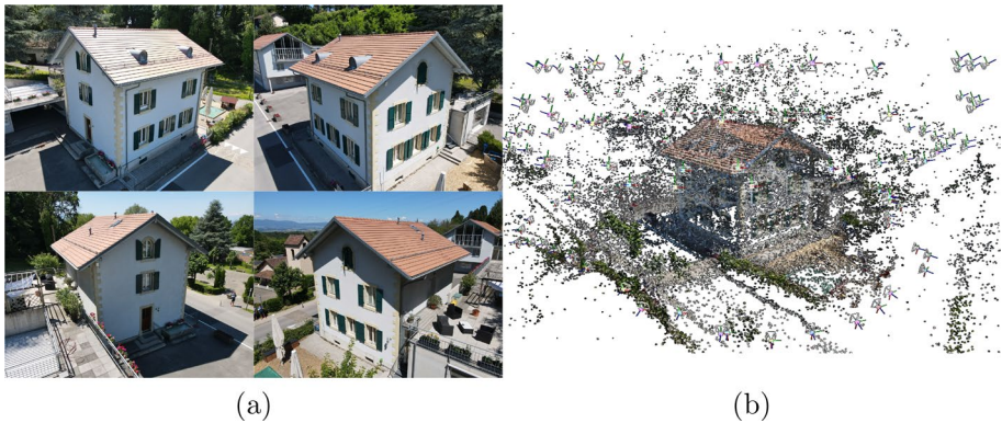
Fig. 3 SfM modeling. a Some images used for SfM processing. b Reconstructed 3D point clouds and camera poses
