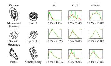
Figure 3: Shape distributions for the example models.
