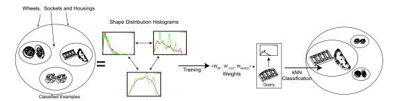
Figure 1: An Overview of our approach: Training with classified examples to classify query models with kNN technique.
