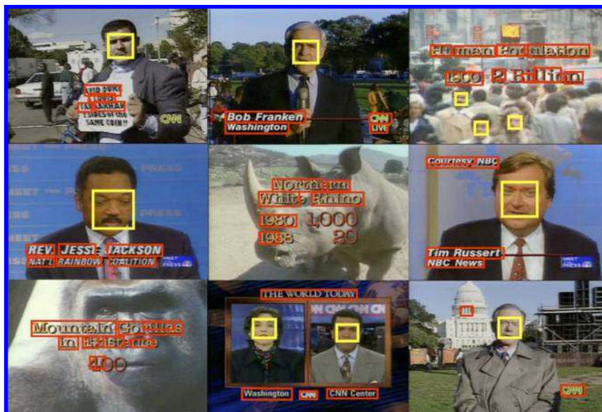
FIGURE 2.7: Red boxes illustrating Informedia automatic text detection against video shots (before subsequent steps to merge smaller detected areas into lines of text), with yellow boxes bounding the detected faces.
