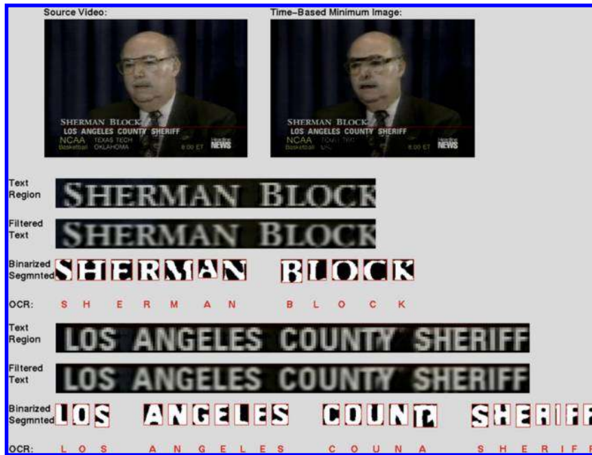
FIGURE 3.7: Example of VOצר process producing incorrect output “COUNA” that could be cleaned up through statistical processing for “Los Angeles <blank> Sheriff” candidates.
