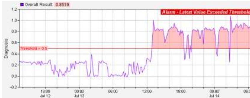
(b) A possible pitch fault has been detected
