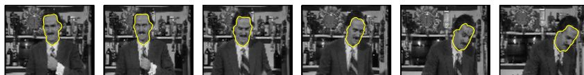
Fig. 6. Model update by tracking. A colour tracker successfully tracks the face over large pose variation and is used to validate proposed updates to the model.
