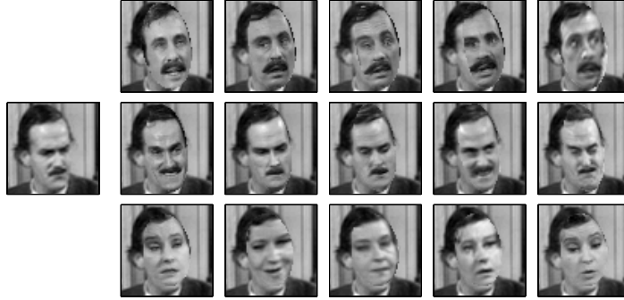
Fig. 4. Face classification based on multiple appearance proposals. The leftmost image is the target, with rows showing proposals rendered from the Manuel, Basil and Sybil models. The task is to decide which proposal to accept, or to reject all.
