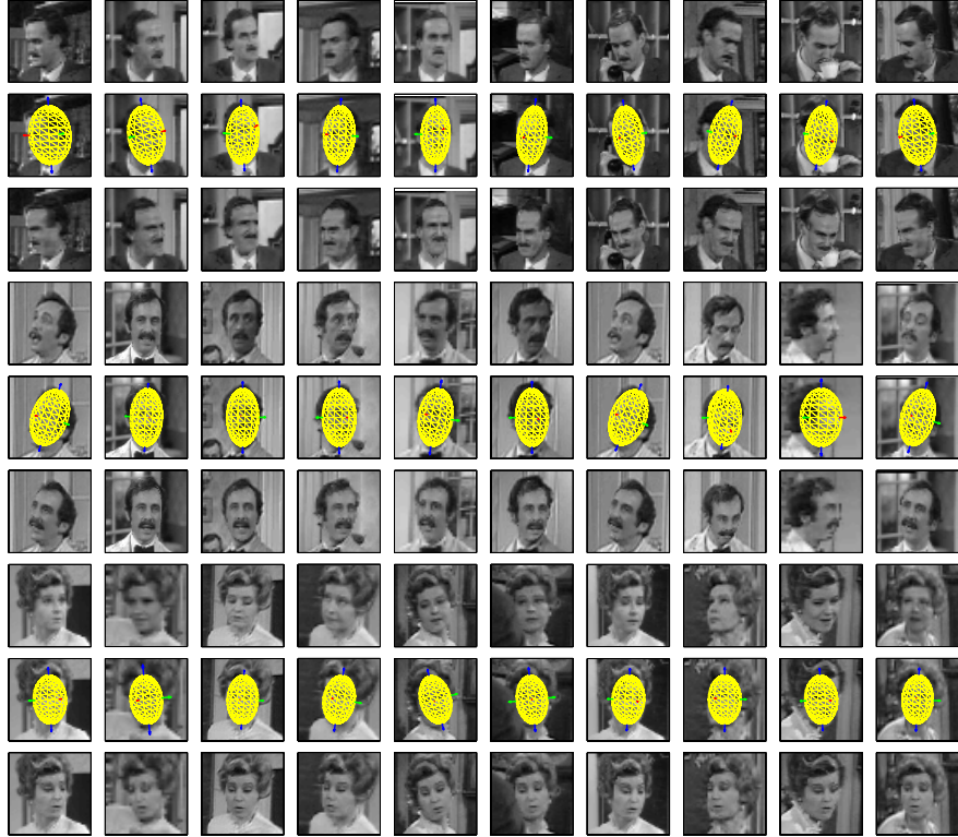
Fig. 3. Pose estimation (best viewed in colour). Top rows show original image, middle rows show ellipsoid overlaid at the estimated pose, bottom rows show overlaid model rendered at the estimated pose.
