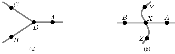
Fig. 3: Two cases that can lead to reconstruction errors. (a) If there is no sample point at bifurcation D, the tree reconstruction algorithm is likely to incorporate both the \overline{AB} and \overline{AC} paths into the final tree, which will result in counting twice the pixels in \overline{AD} when scoring it. This is avoided by introducing an anchor point at D. (b) At a crossover, an anchor point can be used to build either the horizontal \overline{AXB} branch or the vertical \overline{YXZ} one, but not both. This is why we choose to create two anchor points at all potential crossovers.
