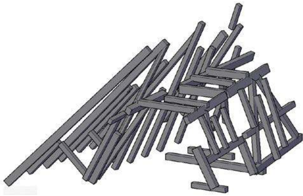
Figure 10: 3-D model containing beams represented by cuboids
