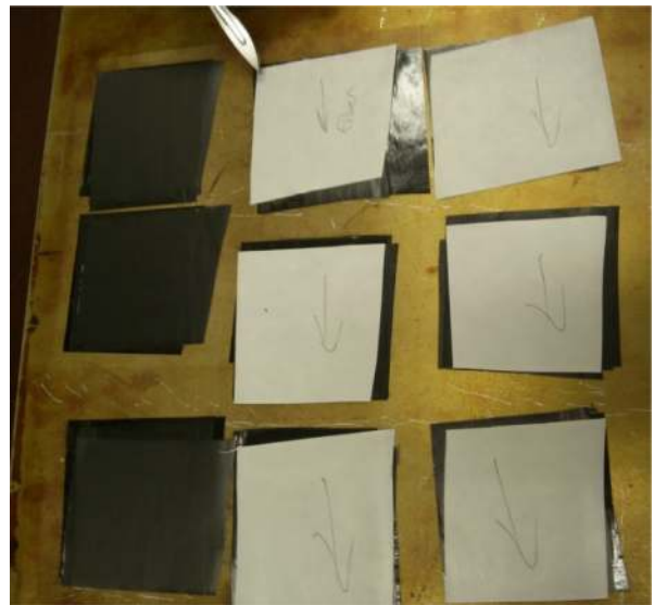
Figure 8. Test samples with indicated fiber direction for peel test.
