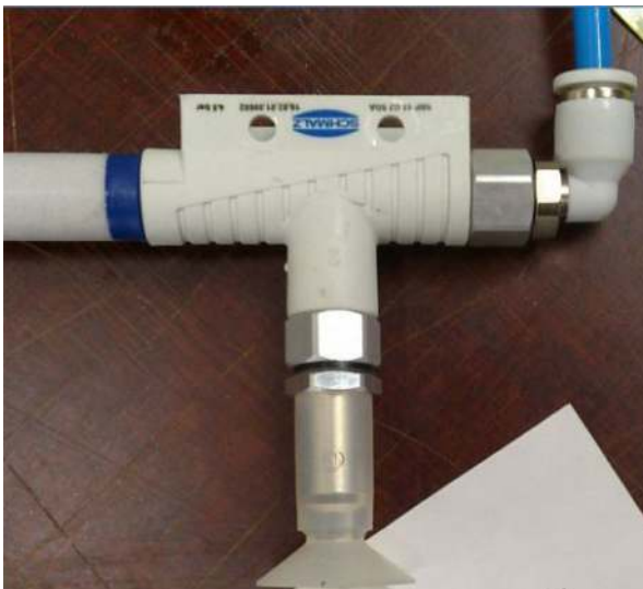
Figure 7. Standard vacuum gripper and ejector.
