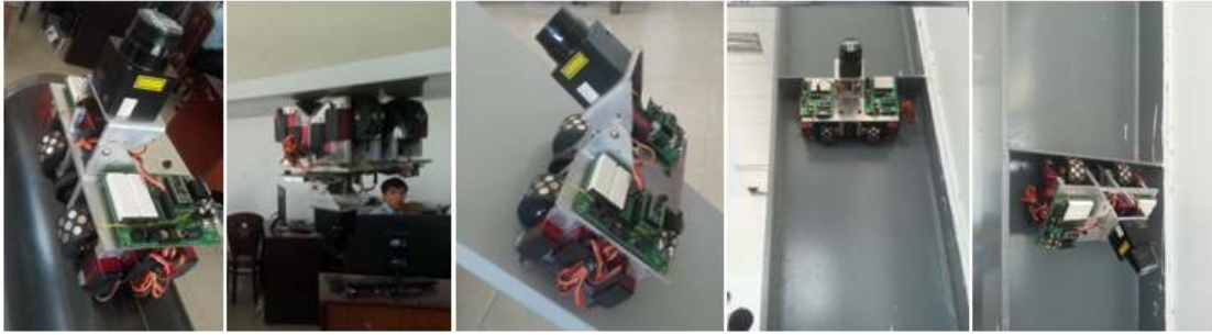
Fig. 13: Adhesion tests on different surfaces under different degrees of inclination.
