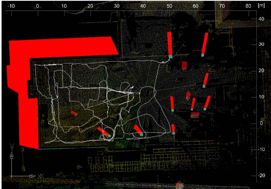
Figure 34 Worker trajectories mapped on laser scan with blind areas taller than 1.5m.
