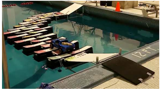
Fig. 17. A bridge of 33 modules spans one corner of the pool, extending 3.7 m \times 2.6 m. A remote controlled car successfully traverses the bridge.
