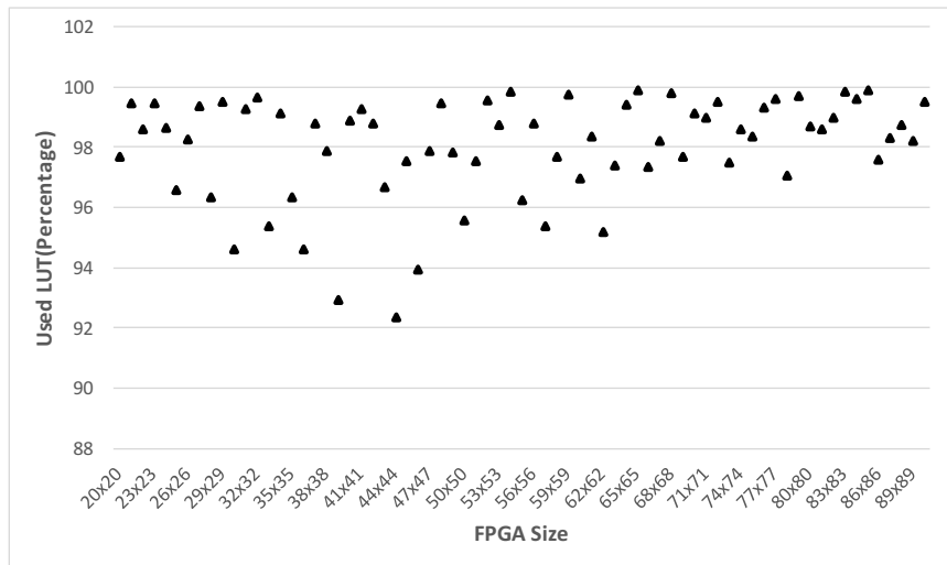
Figure 4.14: LUT usage percentage for Sobel implementations on different FPGA sizes
