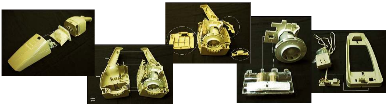
Figure 2. The dissection of a Black & Decker hand held vacuum cleaner.
