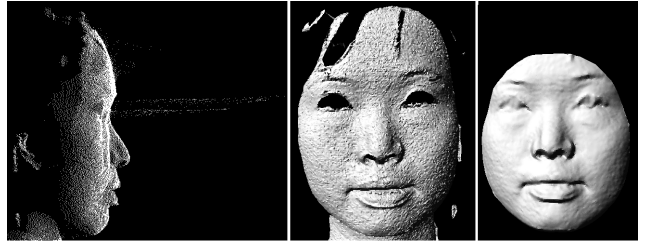
Figure 3. Left: A pointcloud of a face with spikes. Center: Shaded view of the same face after removing the spikes shows that it is noisy. Right: Shaded view of the face after complete preprocessing (i.e. cropping, hole filling, denoising and resampling).
