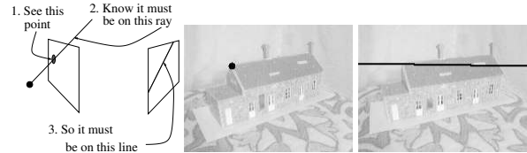
Figure 4: The epipolar line of a point (in the first view) is the image (in the second view) of the ray passing through the point in the first. The two images from the example sequence show a point \mathbf{x} selected in the first generating the line \mathbf{F}\mathbf{x} in the second. The epipolar line of the 2D point in the first view passes through the image of the 3D point in the second view. The \mathbf{F} matrix for these two views was computed automatically by the algorithm described in section 5.1.
