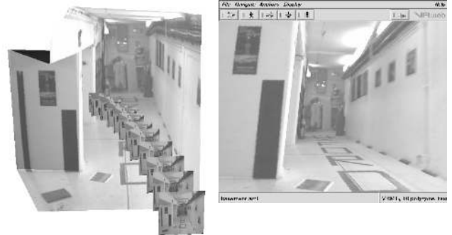
Figure 14: Basement : Texture mapped planar model built from 11 views of the basement sequence. Left: VRML model of the scene with the cameras represented by their image planes (texture mapped with the original images from the sequence). Right: a rendering of the scene from a novel viewpoint different from any in the sequence.
