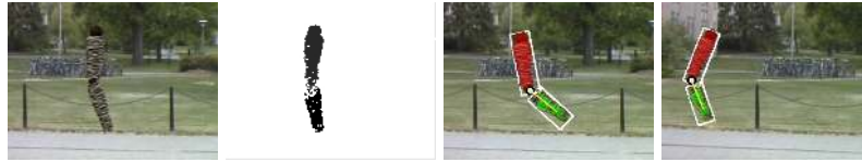
Figure 3: Sequence showing the leg portion of a synthetic walker registered into the world coordinates of actual video footage. The top right image shows the extracted layers with. The bottom two images show two frames from the resulting tracking sequence with the extracted articulated model.
